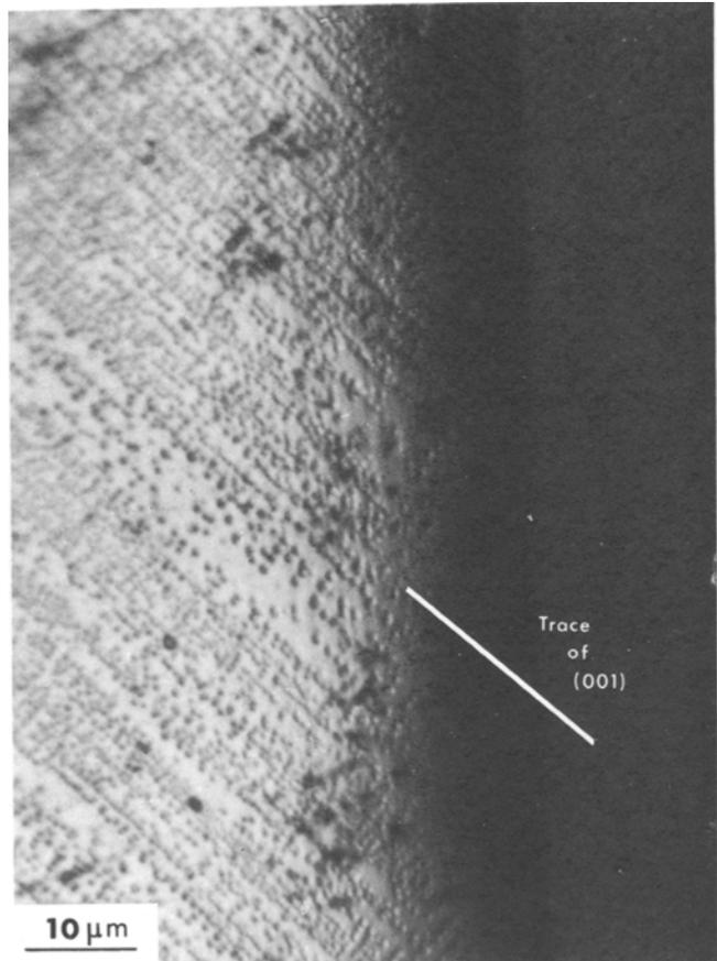
Figure 2 Etch pits (molten KOH, 350° C, 15 min) on sample deformed at 1350° C to 1.5% shear strain. The surface etched is within 5° of (1 1 1) and shows the etch pits aligned along the trace of the (0 0 1) slip plane.
